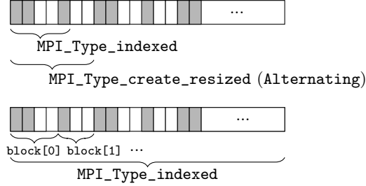
Figure 15: Static Alternating ( \bar{A}\bar{B} ) (top) vs. dynamic Alternating-indexed (bottom) description of the Alternating ( \bar{A}\bar{B} ) layout.
