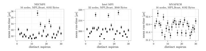
Figure 4: Mean and 95% confidence interval of the time to complete a call to MPI\_Bcast for 30 distinct calls to mpirun. The measurements have been made with different MPI implementations and message sizes on *TUWien*, *VSC-1* and *G5k (Edel)* (from left to right).
