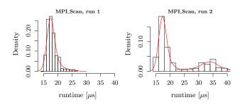
Figure 3: Distribution of the time needed to complete a call to MPI\_Scan (with 250 Bytes and 16 processes) for two distinct calls to mpirun (run 1/run 2). Sample contains 10,000 observations and was taken on *TUWien*.
