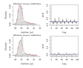
Figure 5: Distribution of runtimes for MPI\_Bcast and the corresponding autocorrelation plot, for the experiments done *without* (top) and *with* random waiting (bottom) times on *TUWien*.
