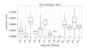
Figure 8: Distribution of the normalized runtimes reported for MPI\_Bcast with various message sizes when running one MPI benchmark 30 times on G5k (Edel).
